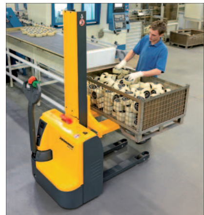
Operating as a lifting table
