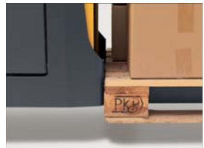
Precise operation with the pallet stop
