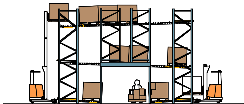
Pallet live storage with order picking tunnel
